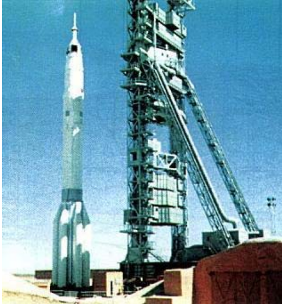
Figure 4. Soviet Soyuz 7K-L1 Spacecraft and UR-500 Launch Vehicle. Source: RKK Energiya.
